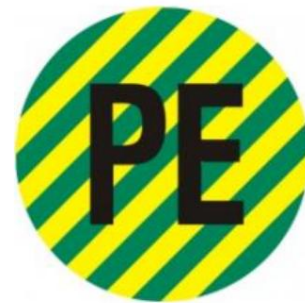
Figure 4: Grounding protection conductor
